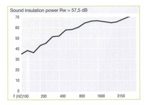
Surface area of test element = 13.40 m<sup>2</sup> L1= Mean level of sound pressure in disturbing chamber
